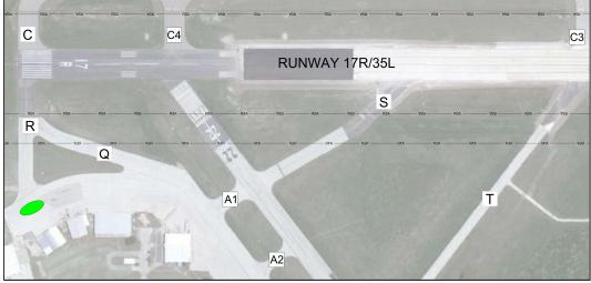
Alternative #1B includes the removal of many of the existing taxiways west of Runway 17R/35L and the redevelopment of a new parallel taxiway system that would mirror the parallel taxiway configuration used on the east side of Runway 17R/35L. The proposed parallel taxiway configuration could be extended further to the south to accommodate additional development in the future. This alternative is shown in **Figure 5-23**.
